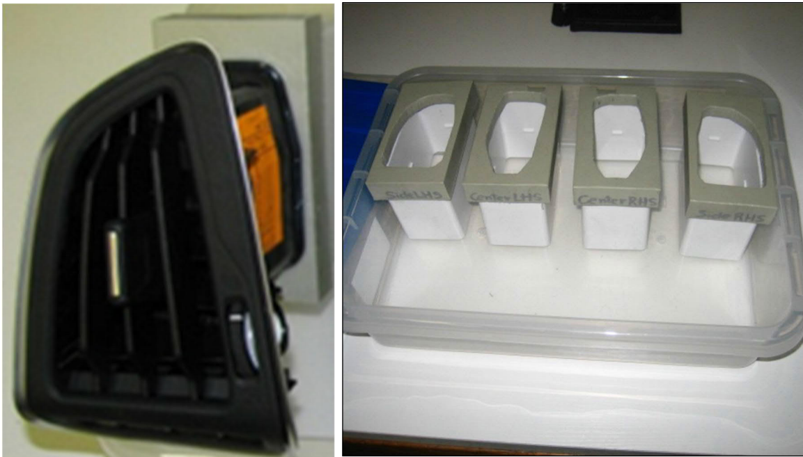
Fig.4.: Air register ( left ), interface elements ( right )
