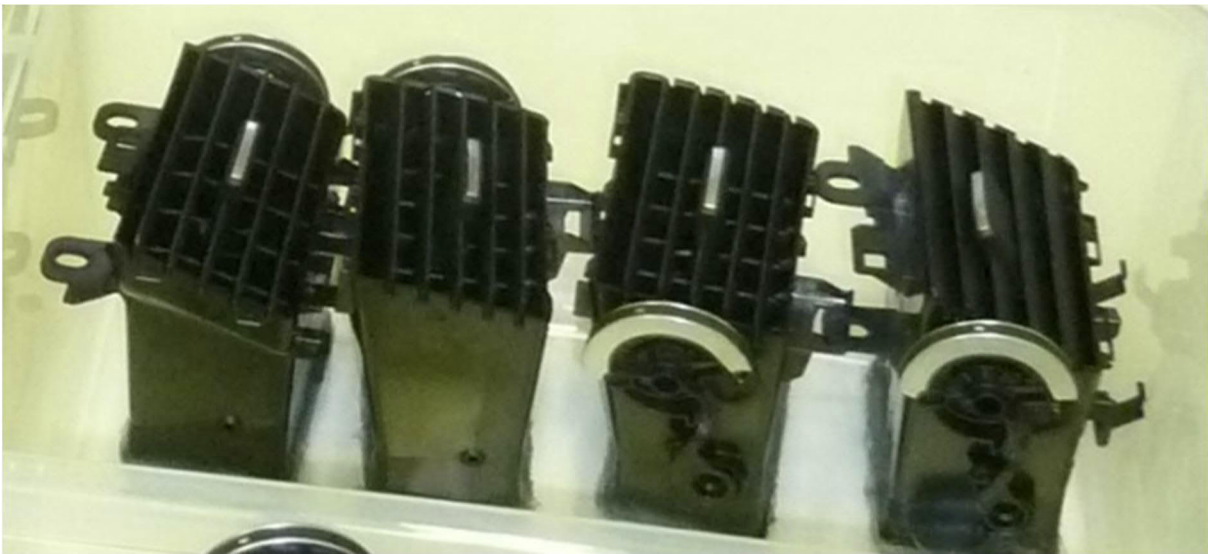
Fig.3.: Air registers of "B" passenger car
